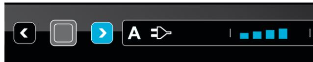
The display of the cooling level begins to flash. Use the directional keys to select the desired cooling level.
