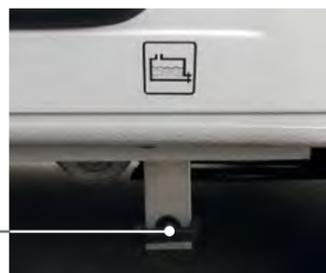
Handle to drain the waste water tank
