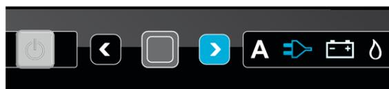
Press the applicable directional key to select the desired energy source.
