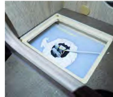
Your mobile home is equipped with a fixed fresh water tank with a capacity of 100 L. The tank is located underneath the left bench, behind the driver's seat.
